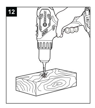
h. To stop the drill/driver, release the trigger switch and allow the tool to come to a complete stop. The electric brake quickly stops the rotation. This feature engages automatically when you release the trigger switch.
