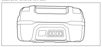
80% - 100% charge 60% - 79% charge  $\bigcirc$   $\bigcirc$   $\bigcirc$   $\bigcirc$ 40% - 59% charge 000 20% - 39% charge 000 Under 20% charge \*\*\* Completely discharged or overloaded  $\textcircled{+} \bigcirc \textcircled{+} \bigcirc$ High/low temperature  $\bigcirc \bigcirc \bigcirc \bigcirc \bigcirc \bigcirc$
