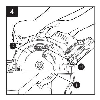
**WARNING:** To avoid possible serious injury, never use the saw when the lower blade guard is not operating correctly. Check the lower blade guard for correct operation before each use. The lower blade guard is operating correctly when it moves freely and instantly returns to the closed position. If the saw is dropped, check the lower blade guard and bumper for damage at all depth settings before using it.
