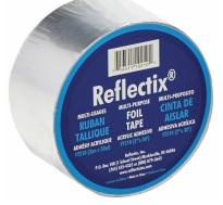
Pressure sensitive tapes require special application procedures for maximum effectiveness. First, the tape must be aligned properly. Make certain there are no wrinkles or folds. After it is applied, the tape should be thoroughly rubbed down with adequate pressure. Plastic applicators should be used to obtain a smooth surface that conforms to the "hills and valleys" of the insulation.
