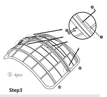
Connecting B to C and D using M8x60mm.
