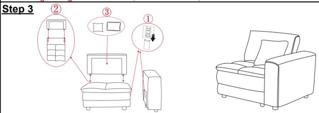
Align backrest with the socket hole and insert it into the back of the sofa, Align the sofa connector with the armrest and install the armrest.
