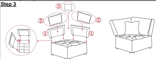
Align backrest with the socket hole and insert it into the back of the sofa
