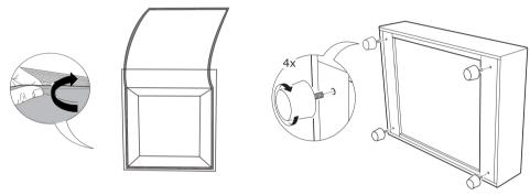
After taking the legs of the sofa out, close the Velcro, then rotate the foot clockwise to install.
