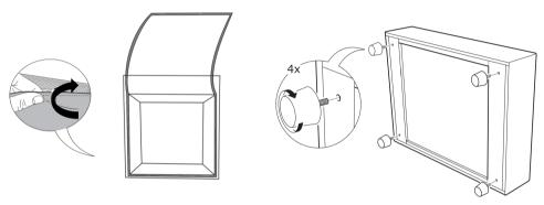
After taking the legs of the sofa out, close the Velcro, then rotate the foot clockwise to install.
