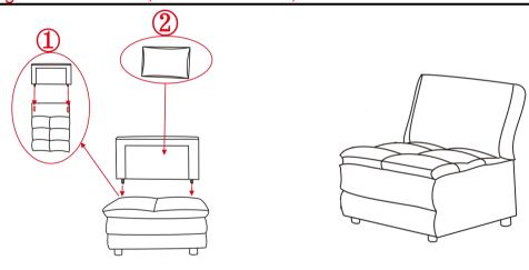
Align backrest with the socket hole and insert it into the back of the sofa
