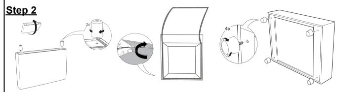
After taking the legs of the sofa out, close the Velcro, then rotate the foot clockwise to install.
