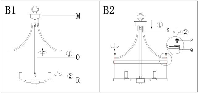
Step B1: Thread the tube (O)onto the bottom of trim(M) .
