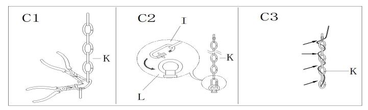
Step C1: By measuring, determine the correct number of links needed for proper hanging height. Using the chain pliers,
