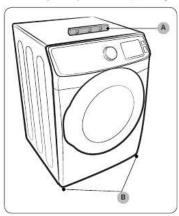
Using a level (A), check if the dryer is level side to side and then front to back. If the dryer is not level, adjust the leveling feet (B) at the bottom of the dryer. Then, check if the dryer is level again.
