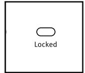
To open the lid after it has been locked, press START/Pause. The lid will unlock once the washer movement has stopped. This may take several minutes if the load was spinning at high speed. Press START/Pause while the lid is closed to resume the cycle.
