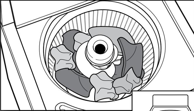
Load garments in loose heaps evenly around basket wall. For best results, do not pack the load tightly. Do not wrap large items such as sheets around the agitator; load them in loose piles around the sides of the basket. Try mixing different-sized items to reduce tangling.
