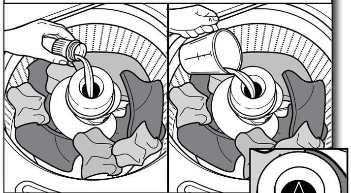
Pour a measured amount of liquid fabric softener into dispenser; always follow manufacturer's directions for correct amount of fabric softener based on your load size.
