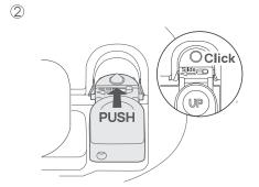
Align the float with the cavities on both sides and push downwards till you hear the "click"
