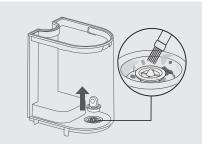
Remove any particles or hair blocking the water valve.
