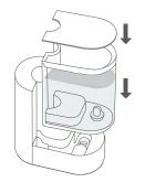
Attach the water tank to the base. replace the top cover.
