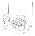
The mineral absorption pads help reduce mineral buildup (scale) inside the humidifier, especially on the heating element.
