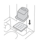
Place the absorption pad and the noise silencer back to the PTC heater.
