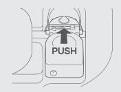
Align the float with the cavities on both sides and push downwards till you hear the "click".
