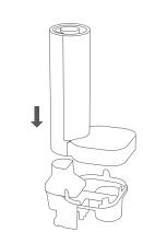
Place the mist tube on top of the hot/cold mist mixer. Make sure the two parts click in place.
