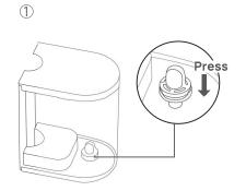
Place the water filter back into the tank. Make sure the water filter clicks in place.
