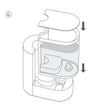
Put the water tank back in place and close the top cover.
