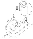
Attach the mist tube to the back of the base.
