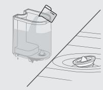
The water valve is not flat or the tank leaks water when refilling.
