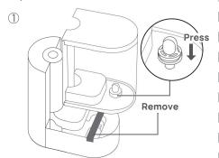
Make sure the water filter is installed correctly and the yellow label has been removed.
