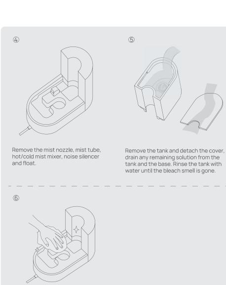
Clean the base with a soft cloth or the included cleaning brush to remove excess of mineral deposits. Make sure all parts are dry before reassembling your humidifier.
