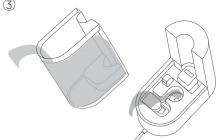
Take out the water tank cover, drain any remaining water from the tank and thé base.
