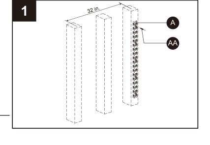
2. With only the top-screw in place, rotate the Post (A) 90-degree in the desired direction. Place a level on the top of the Post (A), that has been rotated 90-degree. Note: Make sure it is level and that the bottom hole of the Post (A) is on-center with the new joist. Mark the spot on the new joist using the bottom hole of the Post (A). Drill a small pilot hole (1/8 in) in this location.
