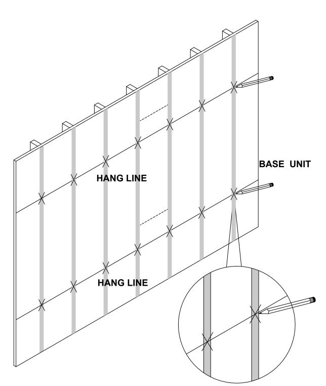
2. Mark locations of studs. On the hang line. Using a stud finder,locate studs to which the unit will be secured.Mark stud locations with a pencil
