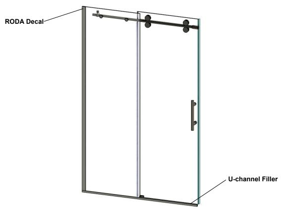
**16** Place large Vinyl Seal [15] on Door Panel [2] so that the vinyl edge sticks out towards the Fixed Glass Panel [1]. Then place smaller 3/8" Vinyl Seal [6] on the handle side of the Door Panel [2] so that the vinyl edge sticks out towards the inside of the shower. (See Example) Use silicone to hold in place.
