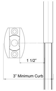
**Note**: Centerline (CL) is a term used to describe the center or mid-point of the unit. The position of the unit centerline can be located anywhere within the width of the threshold, as long as adequate structure exists beneath the centerline for fastening and the outer edges of the unit will not overhang the threshold. The most common unit centerline position is the middle of the threshold.
