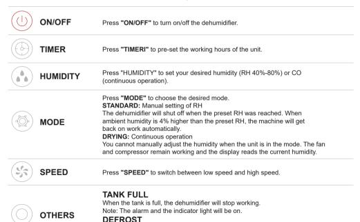
Auto detection of frost and auto defrosting to keep a good performance in dehumidifying. The indicator light will be on until the frost disappears.
