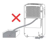
No space between the outlet of hose and the vessel
