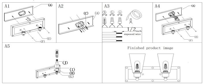
Step A1: Unscrew the ball knobs(F) from back plate(E) then gently remove mounting plate (A)
