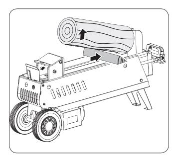
Repeat above procedure with sharper-sloped wood wedge until the log is completely freed.
