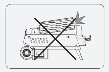
Do not split logs on the upper part of the blade. This could break the blade or damage the machine.
