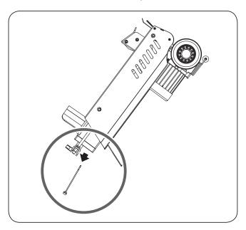
• Tip the log splitter so the motor end is higher than the oil drain plug, and drain oil over a 3- gallon container.
