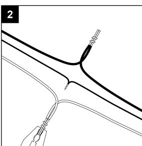
3. Attach wire nuts (AA). Tape wire nuts (AA) and wires together with electrical tape (not included).
