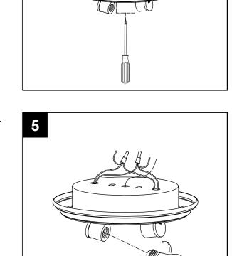
6. Remove knob (H), cap (G), nut (F), rubber ring (D) and washer (C) from the threaded nipple (B). Tighten the threaded nipple (B) into the fixture (A). Place the washer (C), rubber ring (D) and glass shade (E) onto the threaded nipple (B), then secure with nut (F). Place cap (G) onto the threaded nipple (B) and secure with knob (H).
