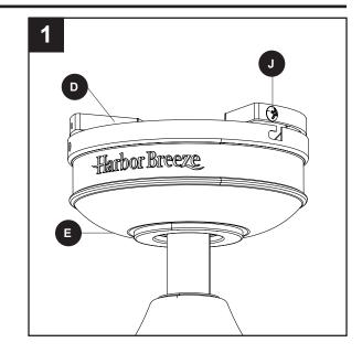
2. Secure the canopy (E) with the mounting bracket screws (J) previously removed (Step 4, page 8). Tighten all mounting bracket screws (J) securely.
