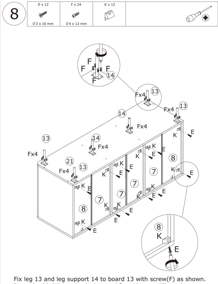
Insert buckle(K) into back slots and fix with screw(E) as shown.
