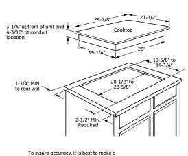
template when cutting the opening in the counter
