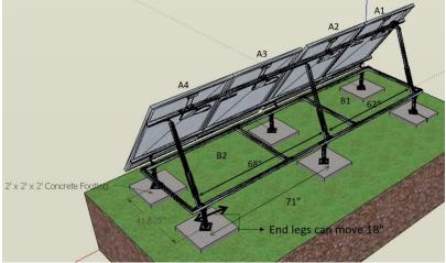
The center legs are fixed. The end legs can move 18" from each end.
