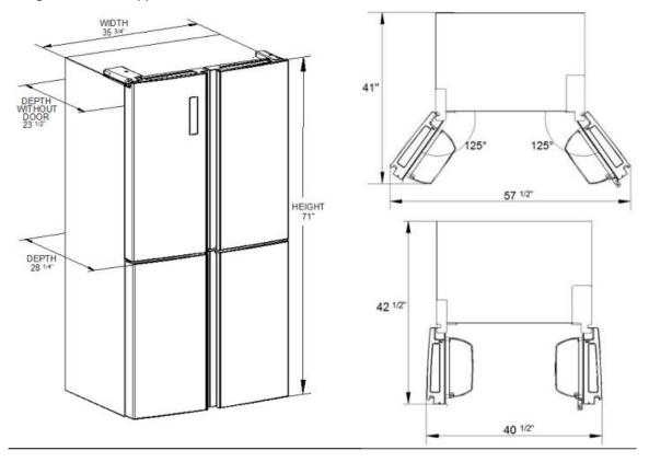
Keep enough clearances between the appliance and its surroundings to ensure the function of the appliance.
