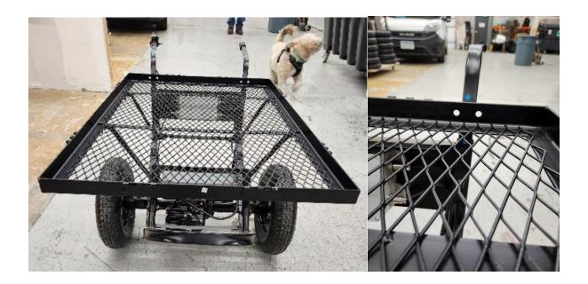
Stand the Deckbarrow up on the dump brace or work from underneath, with the battery removed for access. Center the support brackets to the chassis and tighten.
