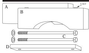
Wood Clamps provide a means for attaching your gate to a post without damaging the post with screws. Please follow these procedures to install a CARDINAL GATE.
