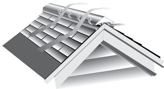
Figure 7-20: A baffled CertainTeed Ridge Vent creates an area of low pressure on both sides of the ridge vent. It literally lifts air out of the attic through both sides of the vent.
