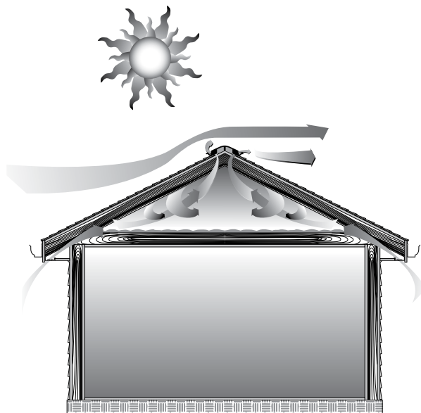
Figure 7-7: Thermal Flow (effect whereby cooler air falls, warmer air rises) and Natural Flow (effect due to wind) come together to ventilate an attic.
