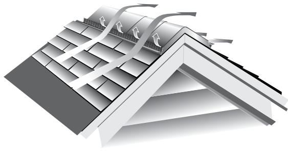
Figure 7-23: An externally baffled vent “pulls” air from the attic through both sides of the vent.
