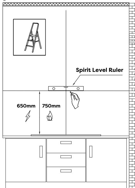
4) Poke the 7 perforated positions on the 1:1 Installation Diagram, then align with the center point of aluminum grease filter on the Installation Diagram with the horizontal line on the wall, then tape the Installation Diagram to the wall, and use a pencil to mark the perforated positions on the wall in the corresponding positions.
