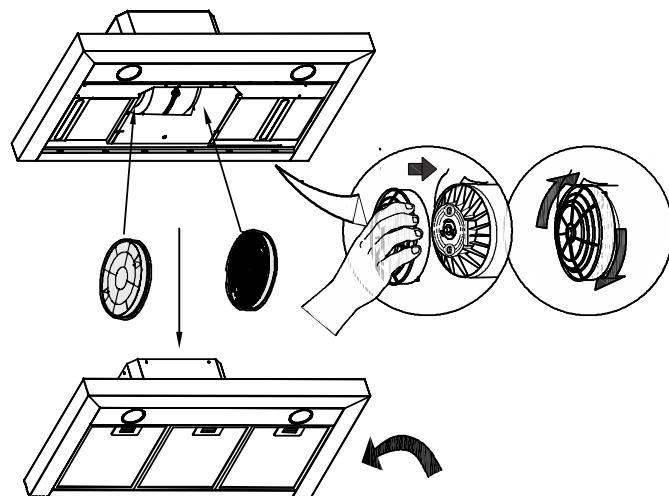
3. If the carbon filter needs to be replaced, please turn it in the anti-clockwise direction.
