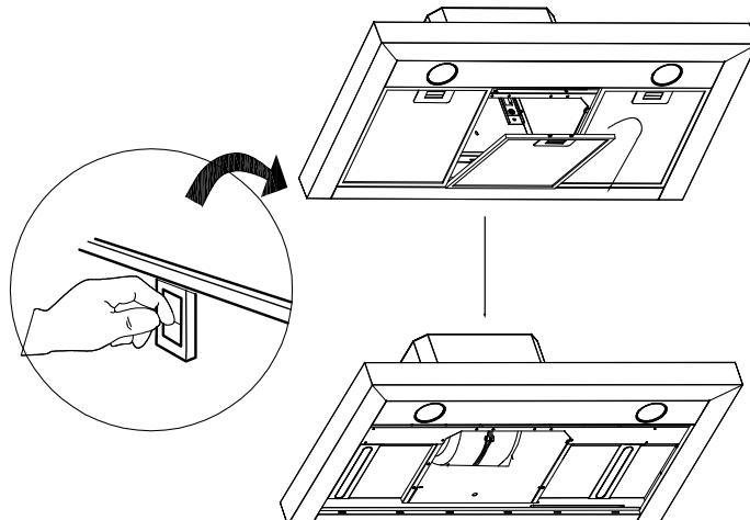
2. Push the LED lamp holder out from the cabinet by hand, or use slotted screwdriver to prize up the LED lamp around the edges, pull out the LED lamp and the wire together.
