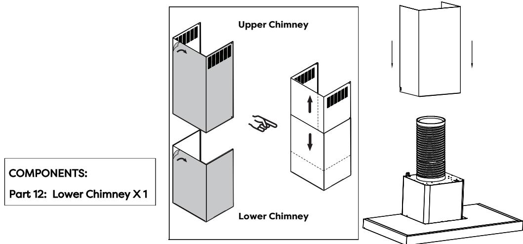
14) Lock the Lower Chimney on the Lower Chimney Bracket by two sides.
