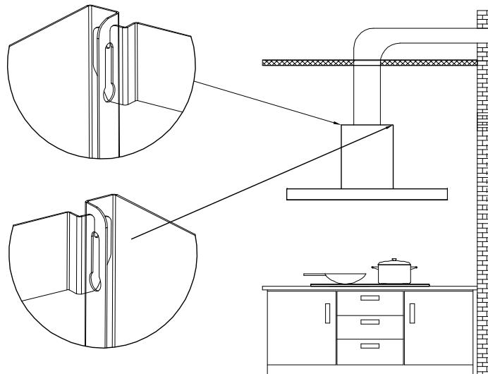
15) Put the Upper Chimney into the Lower Chimney, and then pulled to the height of the Upper Chimney Bracket.
