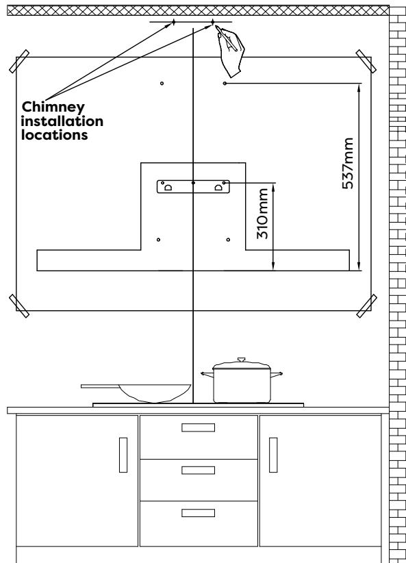
6) Remove the Installation Diagram, drill the holes that have been marked on the wall with an Electric Drill (8mm drill), and hammer the Wall Plug into the wall.
