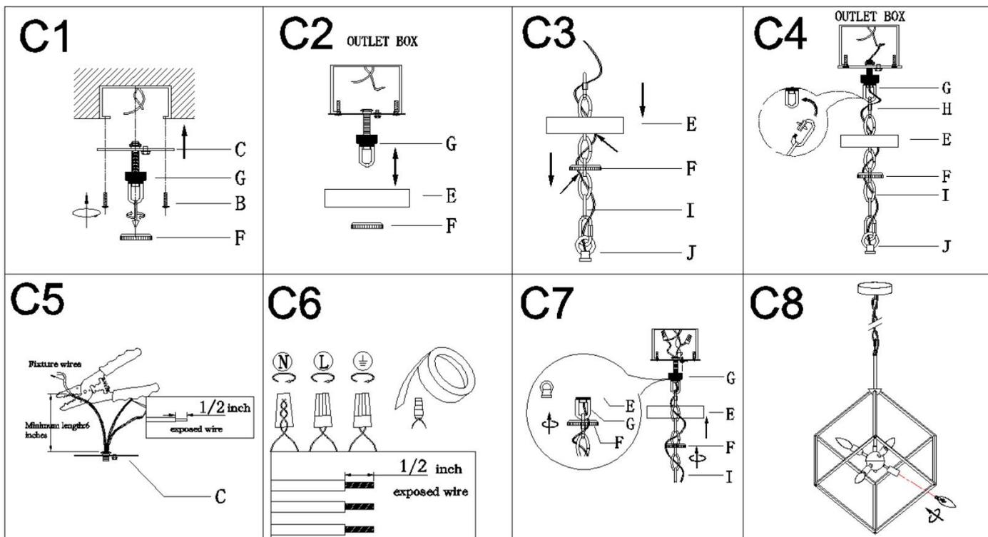
Step C1: Remove collar ring (F) from collar loop (G). Attach single bar (C) to the outlet box with mounting screws (B). **Note: be sure that the side of single bar marked "GND" must face out.**
