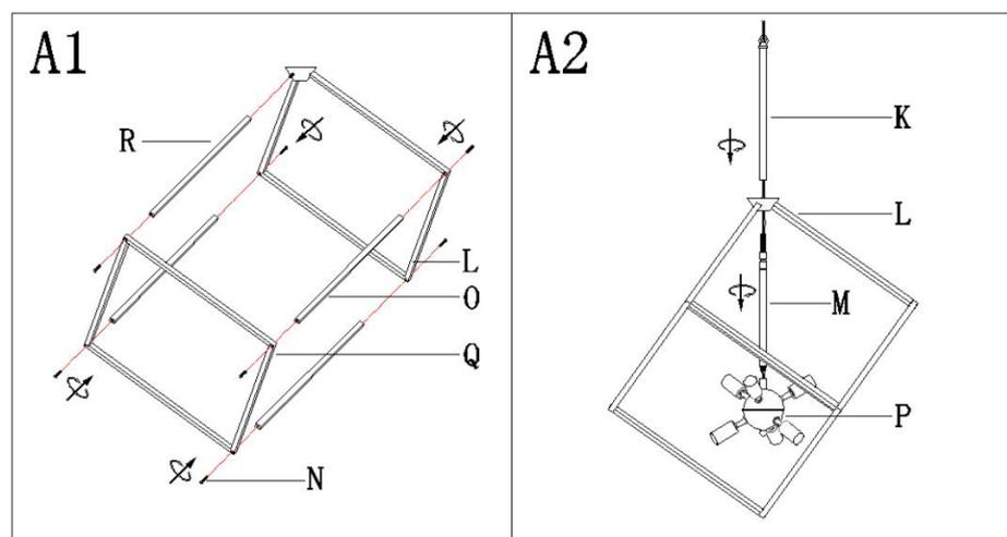
Step A1: Attach upper iron frame (L) and lower iron frame (Q) with longish tubes (O) and shortish tube (R), then secure with screws (N).
