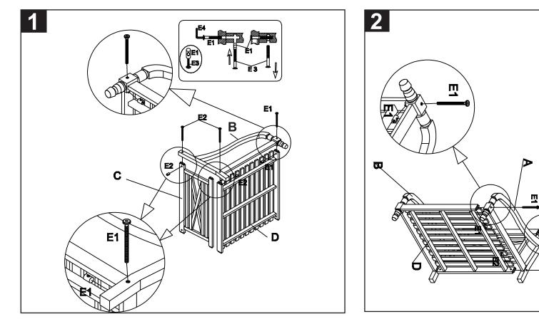
Step1: attach the right side (B) and the back(C) to the seat (D) as shown on the picture by using the Allen bolt (E1) and (E2).Tighten with the Allen key (E4).
