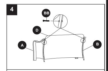
Once all bolts have been installed and hand tightened, go back and tighten firmly.
