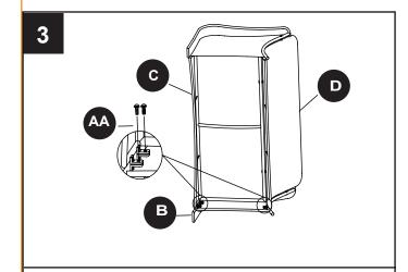
Hand tighten AA. Do not tighten until all bolts have been installed.
