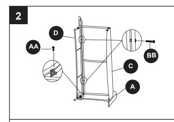
Hand tighten AA and BB. Do not tighten until all bolts have been installed.
