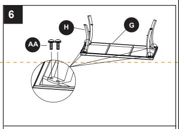
Hand tighten AA. Do not tighten until all bolts have been installed.
