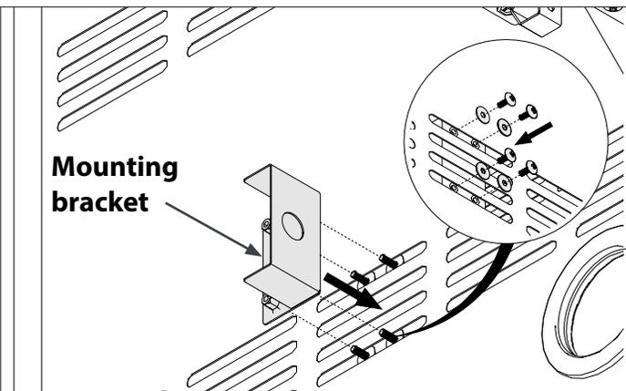
**2** Remove the screws and use for installing the L brackets.
