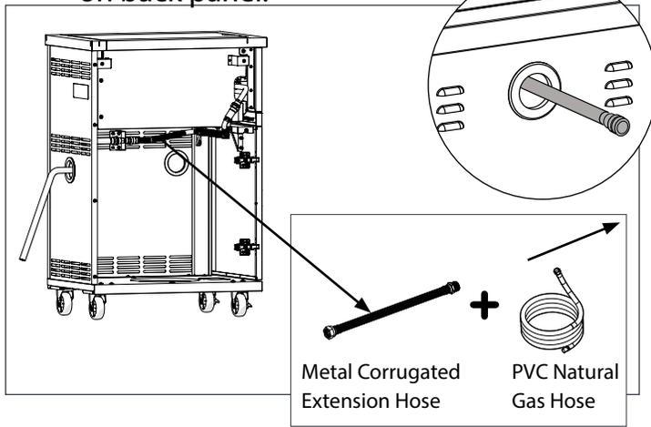
**2** Connect PVC Natural gas hose end to Natural Gas supply using the quick connect fitting.
