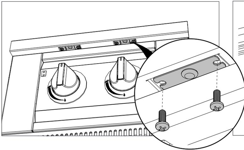
**2** Remove the LED light assembly and disconnect it from the power connector.
