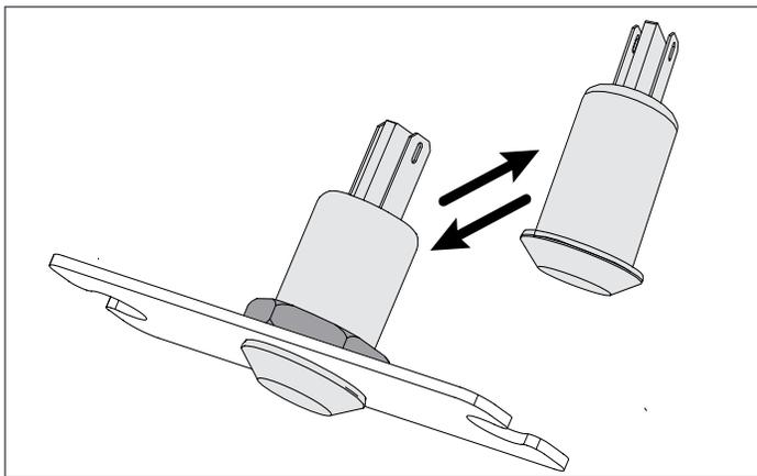
**4** Connect the LED light assembly to the power connector and secure it to the grill with the two screws using Phillips head screw driver.
