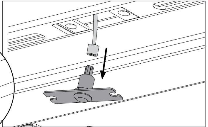
**3** Loosen the lock nut and replace the LED Bulb.
