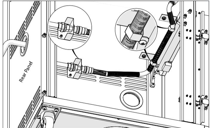
**1** Install Mounting bracket on the cabinet side panel vent slots using Provided washers and Philips screws.
