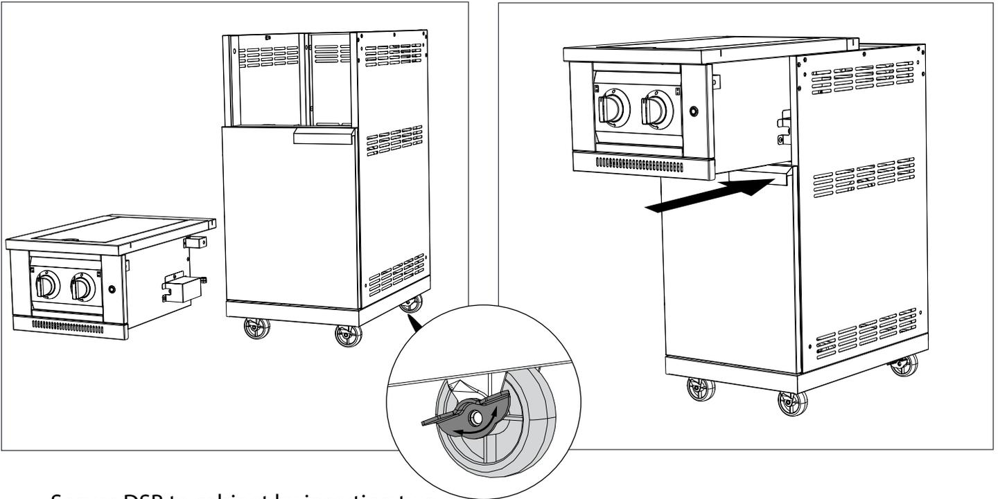
**3** Secure DSB to cabinet by inserting two M6x50mm from the bottom. Flat head screws are provided with the DSB.
