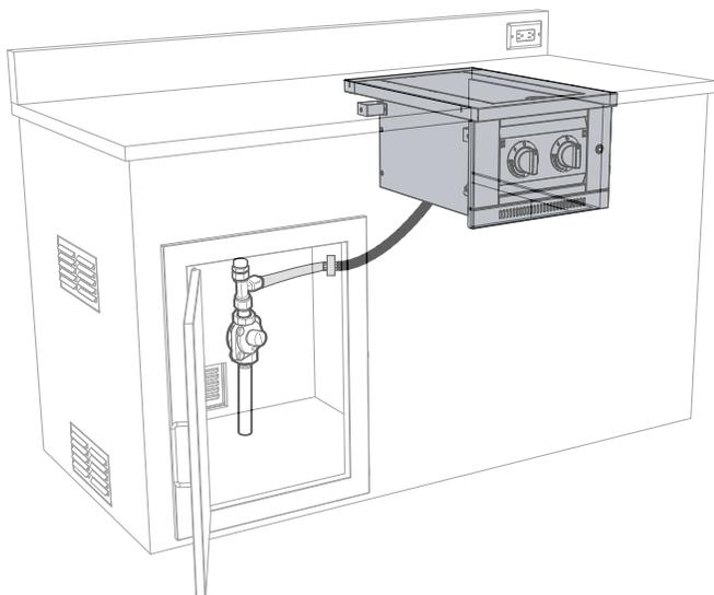
HOSE SHOULD HAVE A SMOOTH SNAKED PATH TO PREVENT KINKS AND PREMATURE FAILURE. PLEASE EXAMINE HOSE AND FITTINGS FOR CRACKS, TEARS, OR WEAR MARKS FROM RUBBING ETC.
