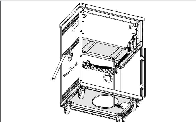
**i** Follow step 1 to 5 for connecting Metal corrugated hose and PVC Natural gas hose together with the help of Mounting bracket, L Bracket and Male adaptor.
