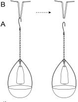
**STEP 2** Slide the Gutter Clip (B) into the rain gutter drain hole.
