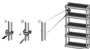
3. Attach wall brackets to a wall stud using appropriate hardware (not included).
