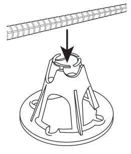
3 No tying is needed to secure bars. Can also be used with remesh.
