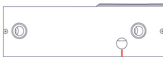
3/4" punchout with Romex connector
