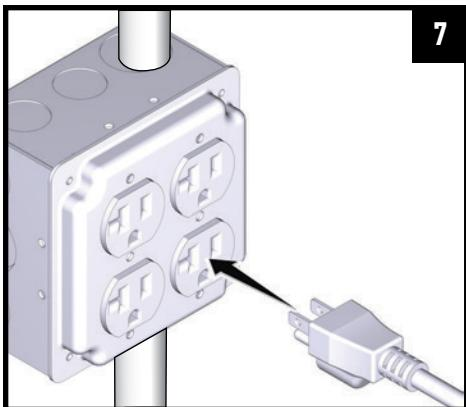
Plug the power adapter into the outlet and mount off the ground using included wall mount bracket. The power supply and device must not be buried or installed where the ambient temperature can exceed 140 deg F (60 deg C) or below 32 deg F (0 deg C).
