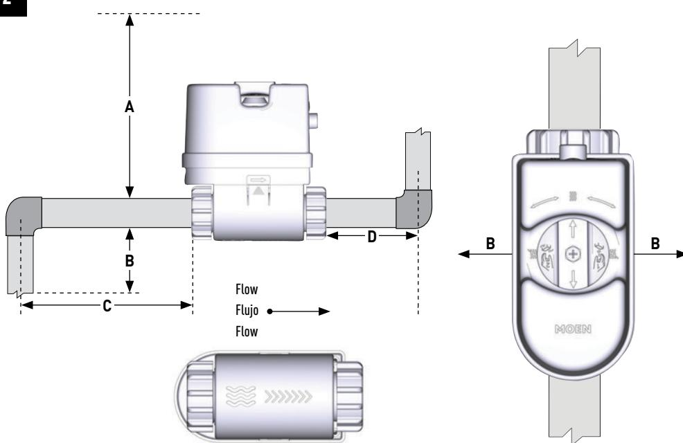
The Clearance needed for the Flo Smart Water Monitor and Shutoff is follows:
