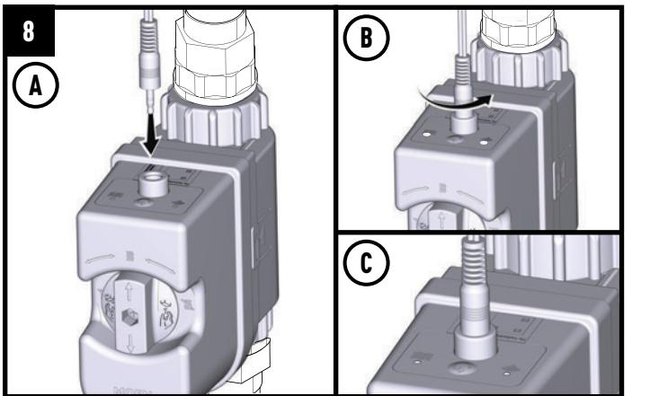
**A.** Plug in the power supply. **B.** Twist and turn while pushing in to create a secure connection. **C.** The status and valve light will turn on and then the valve light will turn green.
