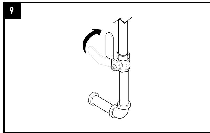
Slowly, open the main water shutoff partially and verify there are not drips or leaks coming from the installation connections. If there are none, slowly open the main water shutoff fully.
