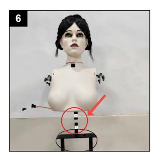
7. Connect the wires from the BODY AND HEAD to both the wires located on the CONTROL BOX.
