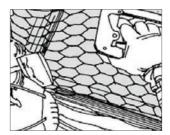
• Mesh Screen or Chicken Wire. Use galvanized chicken wire, nylon mesh or galvanized screen to hold the insulation in place. After the insulation has been pushed into place, staple or nail the mesh or screen to the joist faces.
