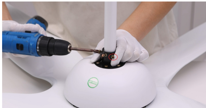
25. Tighten the screws to prevent fan shaking during operation
