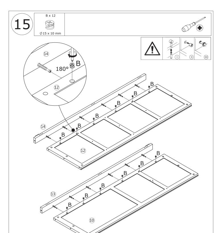
Attach No.14 plate to No.12, and turn cam lock(B) in No.12 plate clockwise to tighten as shown.
