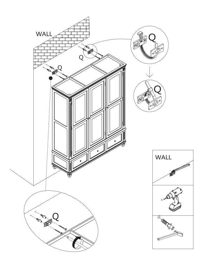
Install anti-tipping device(Q) as shown.
