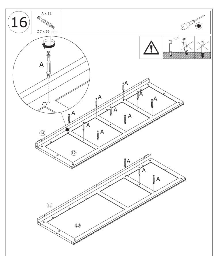
Insert quickfit screw(A) into corresponding holes in No.12 and No.10 plate with a screwdriver as shown.
