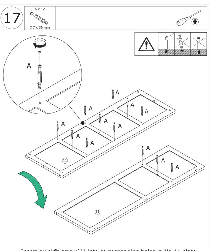
Insert quickfit screw(A) into corresponding holes in No.11 plate with a screwdriver as shown.
