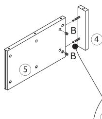
Attach No.4 plate to No.5, and turn cam lock(B) in No.5 plate clockwise to tighten as shown.
