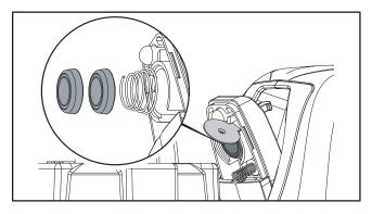
3. Keep the small spring attached to the copper pillar and place the compressed spring back into the bottom of the assembly.
