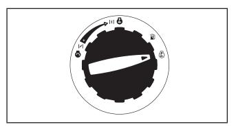
**Important:** Always ensure that the EZ Start dial and fuel lever vent are in the "OFF" position when the generator is not in use.
