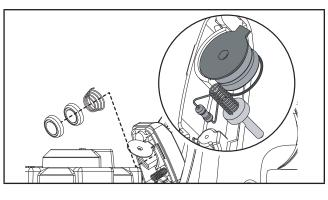
5. Insert the small spring back into the pocket of the upper cover and press the upper cover into place to complete the installation.
