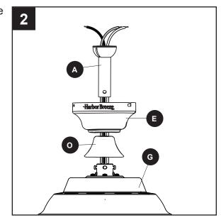
3. Slide the downrod (A) into the yoke of the motor assembly (G), align the holes, then re-install the downrod clip (C) and downrod pin (B). Secure with set screws (Q).
