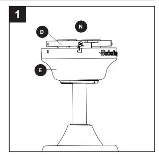
2. Secure the canopy (E) with the mounting bracket screws (N) previously removed (Step 4, page 8). Tighten all mounting bracket screws (N) securely.
