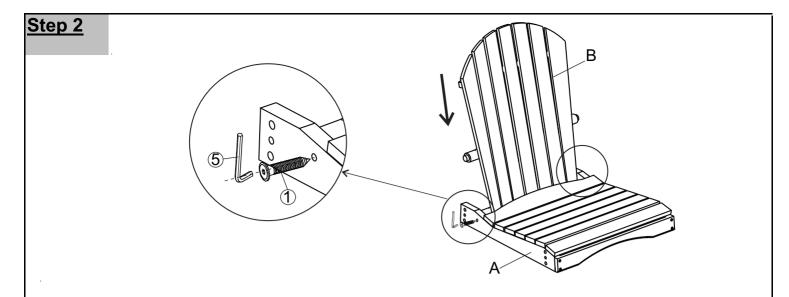
Attach Backrest Panel(B) to Seat Panel(A) using Screws(1) with Allen Key(5) as shown above.
