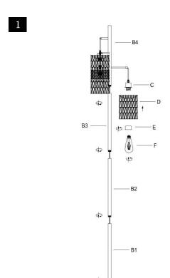
Step 1 Insert Lamp body (B4) into Lamp body (B3) Insert Lamp body (B3) into Lamp body (B2) Insert Lamp body (B2) into Lamp body (B1)
