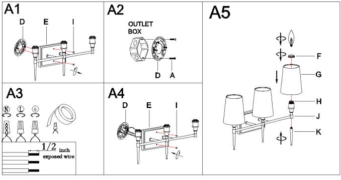
Step A2: Secure mounting plate (D) to outlet box with mounting screws (A).
