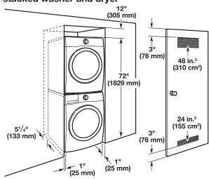
All dimensions show recommended spacing allowed, except for closet door ventilation openings which are the minimum required.
