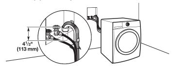
See requirements for floor standpipe drain system.
