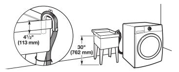
Minimum capacity: 20 gal. (76 L). Top of laundry tub must be at least 30" (762 mm) above floor; install no higher than 96" (2.4 m) from bottom of washer.
