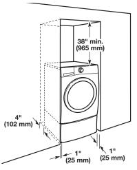
Recessed or closet installation - stacked washer and dryer
