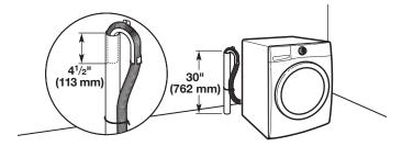
Minimum diameter for a standpipe drain: 2" (51 mm). Minimum carry-away capacity: 17 gal. (64 L) per minute. A 1/4" (6 mm) diameter to 1" (25 mm) diameter Standpipe Adapter Kit is available (Part Number 3363920). Top of standpipe must be at least 30" (762 mm) high; install no higher than 96" (2.4 m) from bottom of washer. If you have an overhead sewer and need to pump higher than 96 inches, a sump pump and associated hardware are needed. See "Alternative Parts".
