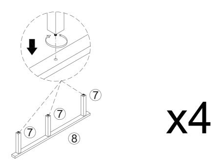
Adjust the leveling feet of the legs 7 to ensure all slats 6 are leveled and staying at the same level.
