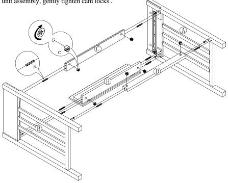
\*\*\*\* Assembling the unit with cam and wood dowels.
