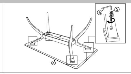
Place the Table top (A) on a soft surface to avoid any scratches or damages to the product and place the Table Leg with the table supporter onto the of table top support with your adult partner.
