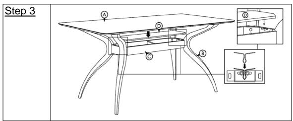
With assistance from your adult partner, stand the Table up. Inspect and make sure all parts are connected, locked and fully secured into position.
