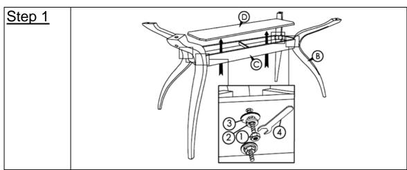
Before assembly, please take out the Table Top supporter (D) as arrow shown. Place the Table Leg (B) into the table supporter corner block. Fix the hanger bolt with Hex Nut ①, Spring Washer ② and Flat Washer ③ using Spanner ④.
