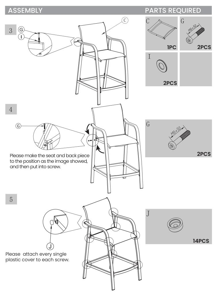
★ If you find stools uneven when assembled, please loosen the 8 screws on the bars, then tighten these screws until stools are adjusted to be even.
