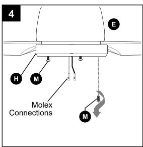
Connect WHITE wire from LED light kit (G) to WHITE wire from motor housing (E). Connect BLACK wire from LED light kit (G) to BLUE (or BLACK) wire from motor housing (E). Make sure molex connections snap together securely.
