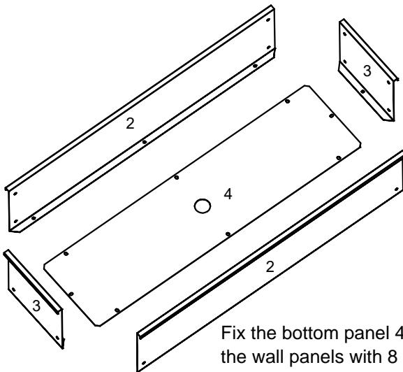
Fix the bottom panel 4# onto the wall panels with 8 pieces F4 screws.
