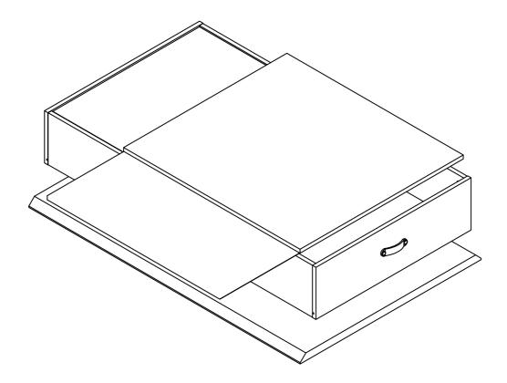
Make sure the unit is rested on a flat surface and does not feel loose or wobbly. If it does, double check all bolts/screws are secured and properly tightened.
